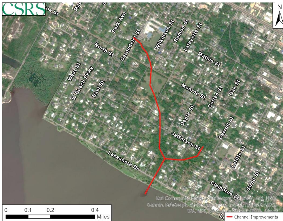
Figure 5-11: Channel Improvement Mitigation Concept
