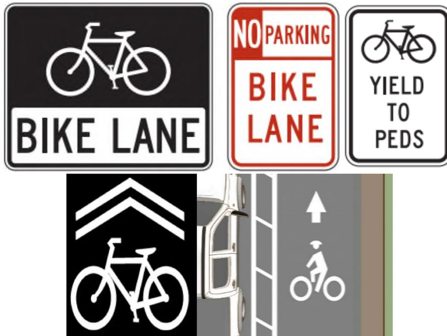
Figure 8-4: Bicycle Pavement Marking and Signage (Source: 2009 MUTCD)
