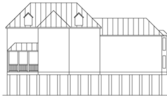
5 Major Elements 4 Minor: Side Porch, Bay Window & 2 Dormers
