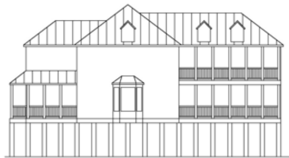
5 Major Elements 5 Minor: Side Porch, Bay Window & 3 Dormers
