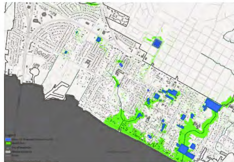
Potential stormwater storage sites identified in the 2023 Mandeville Flood Resilience Strategy by CSRS and Waggoner & Ball
