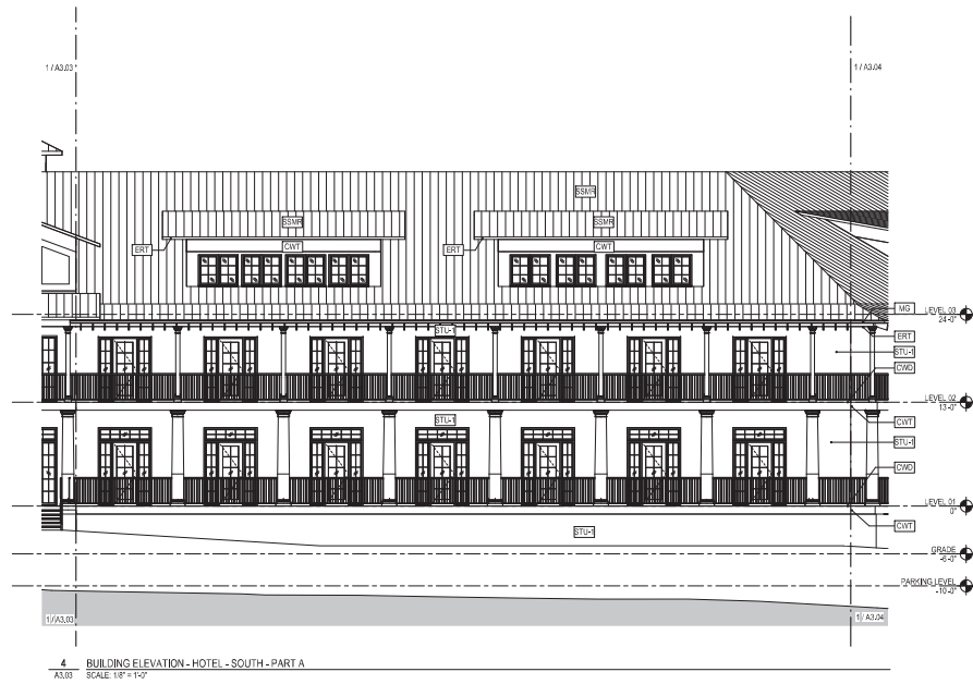
4 BUILDING ELEVATION - HOTEL - SOUTH - PART A SCALE: 1/8" = 1'-0"
