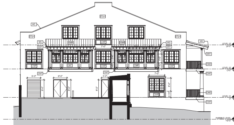
1 BUILDING ELEVATION - HOTEL - WEST A3.05 SCALE: 1/8" = 1'-0"
