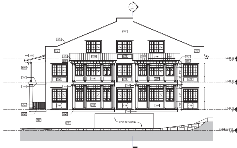
2 BUILDING ELEVATION - HOTEL - EAST A3.05 SCALE: 1/8" = 1'-0"
